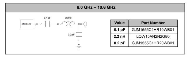
**Figure 3 –** Matching network implemented in the Evaluation Board (Figure 1) for covering the high frequency region from 6.0GHz to 10.6GHz.
