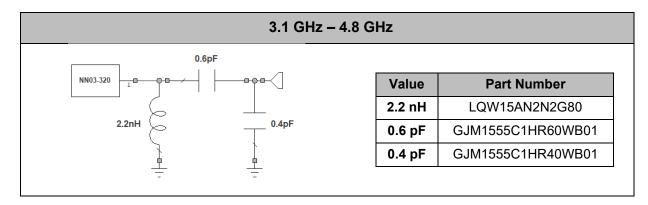
**Figure 2 –** Matching network implemented in the Evaluation Board (Figure 1) for covering the low frequency region from 3.1GHz to 4.8GHz.
