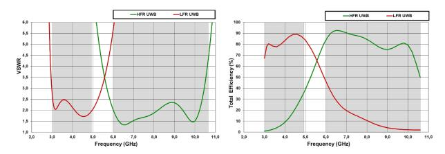
**Figure 4 –** VSWR and total efficiency for the UWB LFR (3.1GHz – 4.8GHz) and for the UWB HFR (6.0GHz – 10.6GHz) from the Evaluation Board (Figure 1 with the matching networks gathered in Figure 2 (LFR UWB) and Figure 3 (HFR UWB), respectively. Simulated results obtained with CST.
