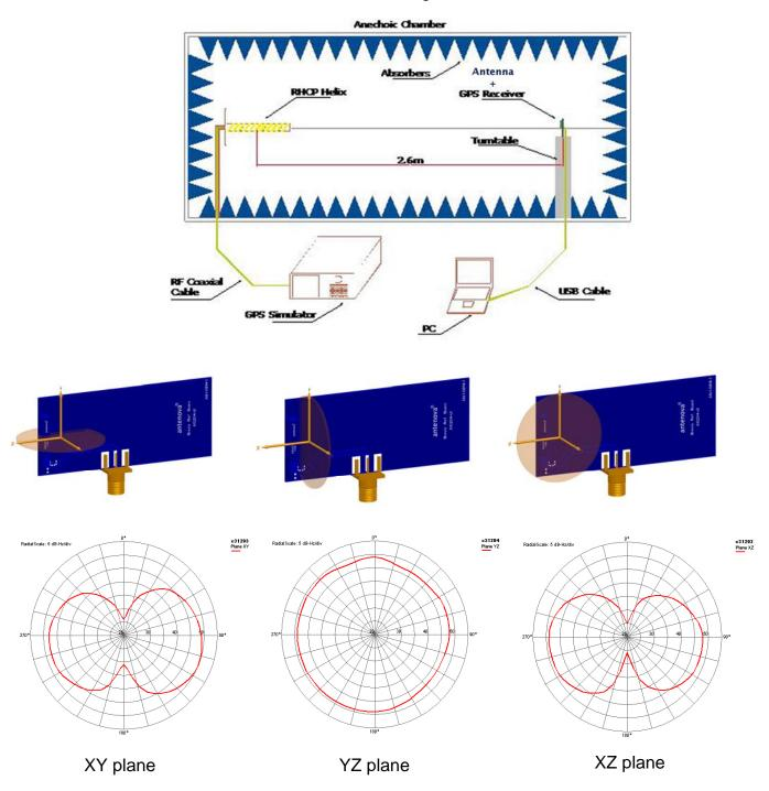
The above plots are CN number in dB.Hz on a scale of 20-50 dB.Hz.
