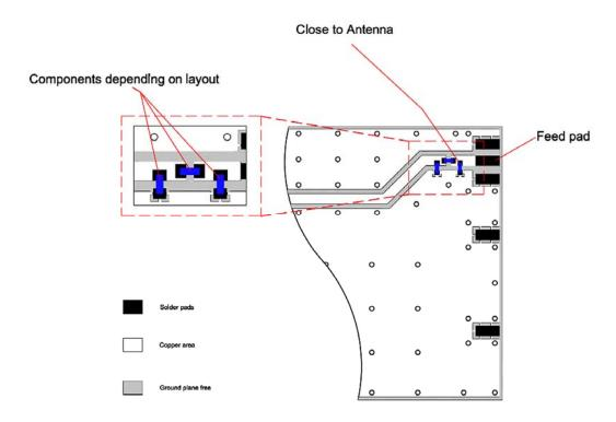
The antenna feed pad and the antenna ground pads are indicated in the drawing above. Additional pads are for mechanical attachment only and should not be grounded.
