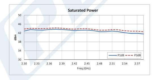
Click the following link (or enter part number in "SEARCH" on website) to obtain additional part information including price, inventory and certifications: S-Band High Power BiDirectional Amplifier, 2.4 GHz to 2.5 GHz 20W Psat, 1 usec Switching, 20dB Tx Gain, Manual T/R Control, SMA PE15B5000
