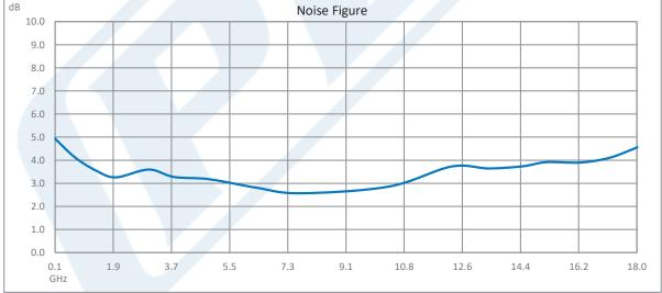
Click the following link (or enter part number in "SEARCH" on website) to obtain additional part information including price, inventory and certifications: Input Protected Low Noise Amplifier, 100 MHz to 18 GHz, 1 Watt RF Input Power, 33 dB Gain, 3.5 dB Noise Figure, 12V, SMA PE15A63020
