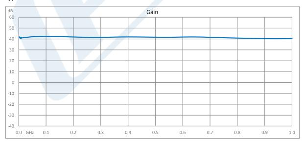
Click the following link (or enter part number in "SEARCH" on website) to obtain additional part information including price, inventory and certifications: Broadband Low Noise Amplifier, 1 KHz to 1000 MHz, 40 dB Gain, 1 dB Noise Figure, +12V, SMA PE15A63012
