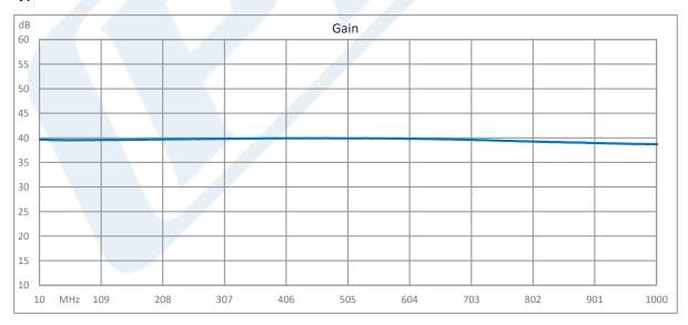
Click the following link (or enter part number in "SEARCH" on website) to obtain additional part information including price, inventory and certifications: 1 dB NF Input Protected Low Noise Amplifier, Operating from 10 MHz to 1 GHz with 40 dB Gain, 17 dBm P1dB and SMA PE15A63001
