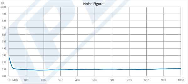
Click the following link (or enter part number in "SEARCH" on website) to obtain additional part information including price, inventory and certifications: 1 dB NF Input Protected Low Noise Amplifier, Operating from 10 MHz to 1 GHz with 30 dB Gain, 17 dBm P1dB and SMA PE15A63000
