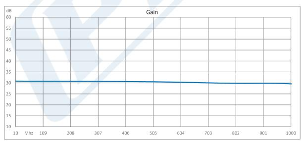
Click the following link (or enter part number in "SEARCH" on website) to obtain additional part information including price, inventory and certifications: 1 dB NF Input Protected Low Noise Amplifier, Operating from 10 MHz to 1 GHz with 30 dB Gain, 17 dBm P1dB and SMA PE15A63000
