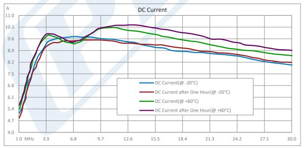
Click the following link (or enter part number in "SEARCH" on website) to obtain additional part information including price, inventory and certifications: 53 dB Gain, 200 Watt Psat, 1.5 MHz to 30 MHz, High Power LDMOS Amplifier, Class AB, Type N Output PE15A5109
