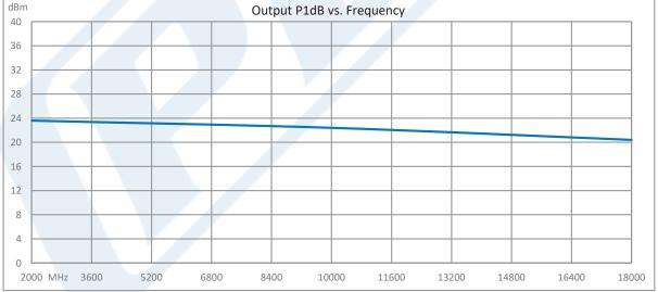
Click the following link (or enter part number in "SEARCH" on website) to obtain additional part information including price, inventory and certifications: Temperature Compensated Low Noise Amplifier, 2 GHz to 18 GHz, 35 dB min Gain, P1dB 22 dBm, SMA, with Heatsink PE15A5106F
