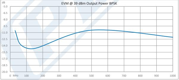
Click the following link (or enter part number in "SEARCH" on website) to obtain additional part information including price, inventory and certifications: High Power GaN Amplifier, 8W Psat, 30 MHz to 2700 MHz, 35 dB Gain, Class AB 12V, SMA PE15A5086
