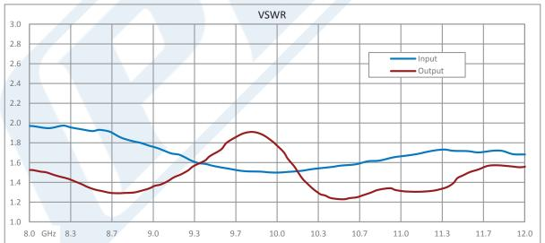
Click the following link (or enter part number in "SEARCH" on website) to obtain additional part information including price, inventory and certifications: 2 Watt P1dB, 8 GHz to 12 GHz, Medium Power Amplifier with Heatsink, SMA, 30 dB Gain, 40 dBm IP3 PE15A5051F
