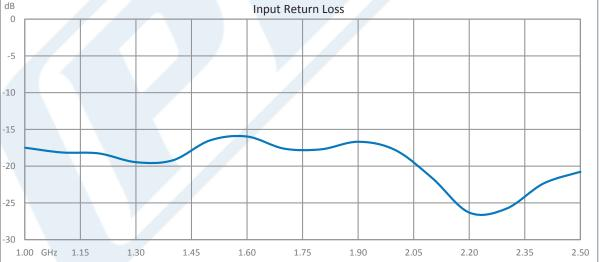
Click the following link (or enter part number in "SEARCH" on website) to obtain additional part information including price, inventory and certifications: 44 dB Gain, 10 Watt Psat, 1 GHz to 2.5 GHz, High Power GaAs Amplifier, SMA Input, SMA Output, 46 dBm IP3, Class A/AB PE15A5036
