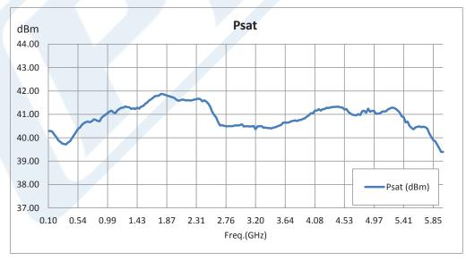
Click the following link (or enter part number in "SEARCH" on website) to obtain additional part information including price, inventory and certifications: 60 dB Gain, 10 Watt Psat, 100 MHz to 6 GHz, High Power GaN Amplifier, SMA Input, SMA Output, 10 dB NF PE15A5027
