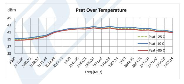
Click the following link (or enter part number in "SEARCH" on website) to obtain additional part information including price, inventory and certifications: 55 dB Gain, 14 Watt P1dB, 2.3 GHz to 2.7 GHz, High Power Amplifier, SMA Input, SMA Output, 53 dBm IP3 PE15A5018
