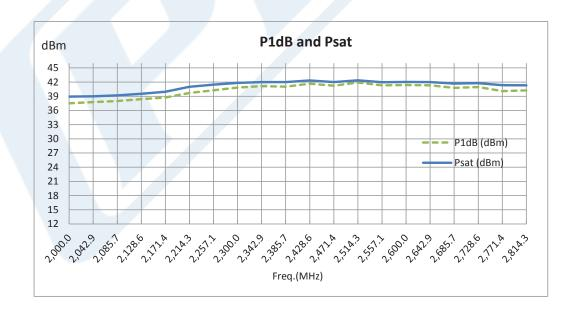
Click the following link (or enter part number in "SEARCH" on website) to obtain additional part information including price, inventory and certifications: 55 dB Gain, 14 Watt P1dB, 2.3 GHz to 2.7 GHz, High Power Amplifier, SMA Input, SMA Output, 53 dBm IP3 PE15A5018
