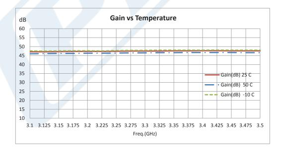
Click the following link (or enter part number in "SEARCH" on website) to obtain additional part information including price, inventory and certifications: 47 dB Gain, 20 Watt P1dB, 3.1 GHz to 3.5 GHz, High Power Amplifier, SMA Input, SMA Output, 3.5 dB NF PE15A5003
