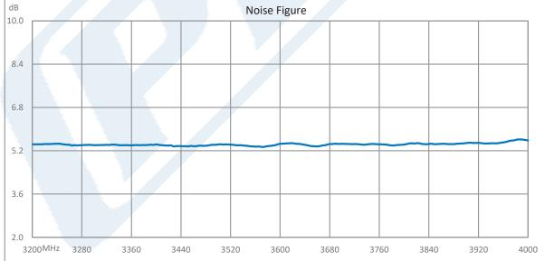
Click the following link (or enter part number in "SEARCH" on website) to obtain additional part information including price, inventory and certifications: 1.5 Watt P1dB, 3.2 GHz to 4 GHz, Medium Power GaAs Amplifier with Heatsink, 35 dB Gain, 42 dBm IP3 and SMA PE15A4076
