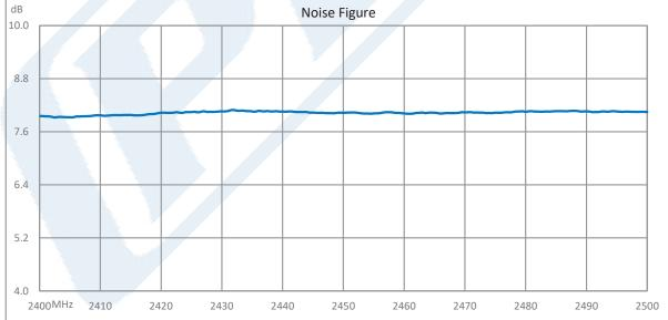
Click the following link (or enter part number in "SEARCH" on website) to obtain additional part information including price, inventory and certifications: 2 Watt P3dB, 2.4 GHz to 2.5 GHz, Medium Power GaAs Amplifier with Heatsink, 31 dB Gain, 43 dBm IP3 and SMA PE15A4075
