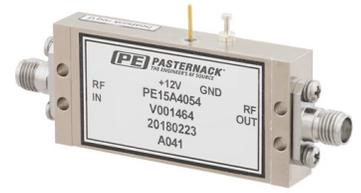
1 Watt P1dB, 2 GHz to 8 GHz, Medium Power Amplifier, SMA, 38 dB Gain, 5.5 dB NF
