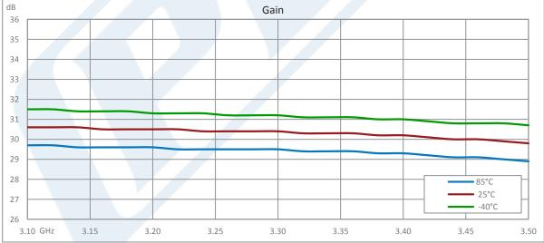
Click the following link (or enter part number in "SEARCH" on website) to obtain additional part information including price, inventory and certifications: 1 Watt P1dB, 3.1 GHz to 3.5 GHz, Medium Power Broadband Amplifier, 30 dB Gain, 4.5 dB NF, SMA PE15A4046
