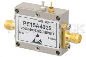
1 Watt P1dB, 820 MHz to 960 MHz, Medium Power GaAs Amplifier, SMA Input, SMA Output, 15 dB Gain, 46 dBm IP3, 2 dB NF
