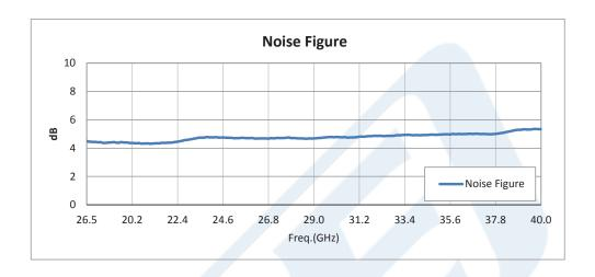
Click the following link (or enter part number in "SEARCH" on website) to obtain additional part information including price, inventory and certifications: 20 dBm P1dB, 26.5 GHz to 40 GHz, Medium Power Broadband Amplifier, 30 dB Gain, 6 dB NF, 2.92mm PE15A4022
