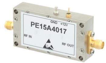
1 Watt P1dB, 30 MHz to 3 GHz, Medium Power GaAs Amplifier, SMA Input, SMA Output, 27 dB Gain, 39 dBm IP3
