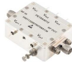
5 Watt Psat, 3.5 GHz to 7 GHz, High Power GaAs Amplifier, SMA, 26 dB Gain, 45 dBm IP3, 11 dB NF
