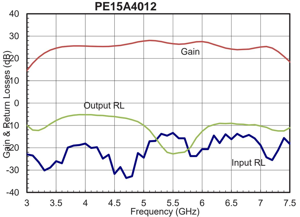
Click the following link (or enter part number in "SEARCH" on website) to obtain additional part information including price, inventory and certifications: [5 Watt Psat, 3.5 GHz to 7 GHz, High Power GaAs Amplifier, SMA, 26 dB Gain, 45 dBm IP3, 11 dB NF PE15A4012](#)
