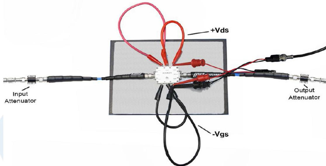
4. Apply the -Vgs voltage -1.0 Volts (Always apply -Vgs first).
