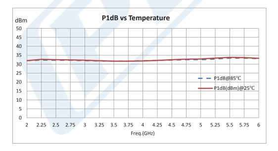
Click the following link (or enter part number in "SEARCH" on website) to obtain additional part information including price, inventory and certifications: 44 dB Gain, 1 Watt, 2 GHz to 6 GHz, Broadband High Gain Amplifier, 39 dBm IP3, 5 dB NF, SMA PE15A3503
