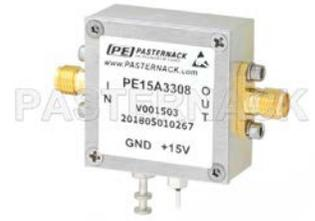
4 dB NF, 12 dBm P1dB, 0.01 MHz to 3 GHz, Low Noise Broadband Amplifier, 16 dB Gain, SMA
