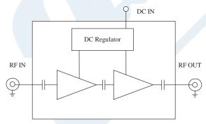
Click the following link (or enter part number in "SEARCH" on website) to obtain additional part information including price, inventory and certifications: 3.5 dB NF, 13.5 dBm P1dB, 26.5 GHz to 40 GHz, Low Noise Broadband Amplifier, 22 dB Gain, 2.92mm PE15A3261
