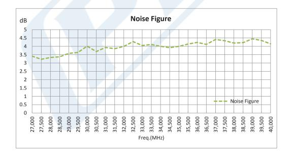
Click the following link (or enter part number in "SEARCH" on website) to obtain additional part information including price, inventory and certifications: 3.5 dB NF, 13.5 dBm P1dB, 26.5 GHz to 40 GHz, Low Noise Broadband Amplifier, 22 dB Gain, 2.92mm PE15A3261
