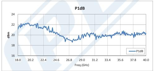
Click the following link (or enter part number in "SEARCH" on website) to obtain additional part information including price, inventory and certifications: 20 dBm P1dB, 18 GHz to 40 GHz, Medium Power Broadband Amplifier, 30 dB Gain, 6.5 dB NF, 2.92mm PE15A3025
