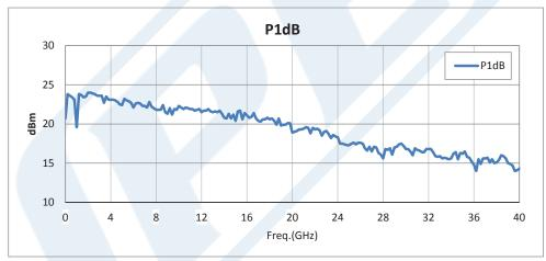
Click the following link (or enter part number in "SEARCH" on website) to obtain additional part information including price, inventory and certifications: 20 dBm P1dB, 30 MHz to 40 GHz, Medium Power Broadband Amplifier, 25 dB Gain, 6 dB NF, 2.92mm PE15A3023
