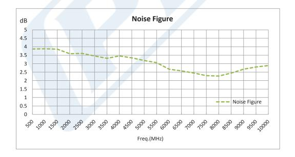
Click the following link (or enter part number in "SEARCH" on website) to obtain additional part information including price, inventory and certifications: 25 dBm P1dB, 500 MHz to 10 GHz, Medium Power Broadband Amplifier, 32 dB Gain, 33 dBm IP3, 3 dB NF, SMA PE15A3005
