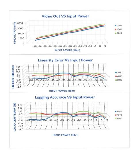
Click the following link (or enter part number in "SEARCH" on website) to obtain additional part information including price, inventory and certifications: 2 GHz to 6 GHz, Log Amplifier, 40 mV/dB Log Slope, 75 dBm Log Range, SMA PE15A2001
