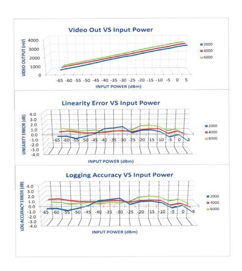
Click the following link (or enter part number in "SEARCH" on website) to obtain additional part information including price, inventory and certifications: 2 GHz to 6 GHz, Log Amplifier, 40 mV/dB Log Slope, 75 dBm Log Range, SMA PE15A2001
