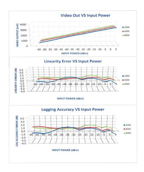
Click the following link (or enter part number in "SEARCH" on website) to obtain additional part information including price, inventory and certifications: 2 GHz to 6 GHz, Log Amplifier, 40 mV/dB Log Slope, 75 dBm Log Range, SMA PE15A2001
