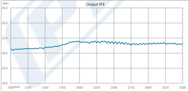
Click the following link (or enter part number in "SEARCH" on website) to obtain additional part information including price, inventory and certifications: 1.0 dB NF Low Noise Amplifier, Operating from 1 GHz to 3.5 GHz with 43 dB Gain, 18 dBm P1dB and SMA PE15A1089
