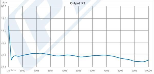
Click the following link (or enter part number in "SEARCH" on website) to obtain additional part information including price, inventory and certifications: 3.2 dB NF Low Noise Amplifier, Operating from 10 MHz to 10 GHz with 37 dB Gain, 15 dBm P1dB and SMA PE15A1088
