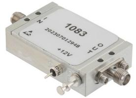
1.4 dB NF Low Noise Amplifier, Operating from 10 MHz to 1 GHz with 30 dB Gain, 29 dBm P1dB and SMA
