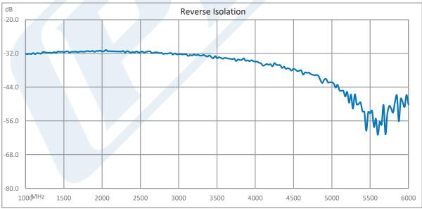
Click the following link (or enter part number in "SEARCH" on website) to obtain additional part information including price, inventory and certifications: 1.0 dB NF Low Noise Amplifier, Operating from 1 GHz to 6 GHz with 18 dB Gain, 18.5 dBm P1dB and SMA PE15A1080
