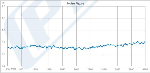
Click the following link (or enter part number in "SEARCH" on website) to obtain additional part information including price, inventory and certifications: 0.7 dB NF Low Noise Amplifier, Operating from 600 MHz to 4200 MHz with 21 dB Gain, 16 dBm P1dB and SMA PE15A1079
