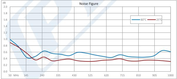
Click the following link (or enter part number in "SEARCH" on website) to obtain additional part information including price, inventory and certifications: 36 dBm IP3, 18 dBm P1dB, 50 MHz to 1,000 MHz, Low Noise Amplifier, 19 dB Gain, SMA PE15A1014
