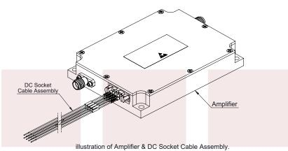
Illustration of Amplifier & DC Socket Cable Assembly Cable Assembly model PE15J000 sold separately (Picture shown for Reference Only)
