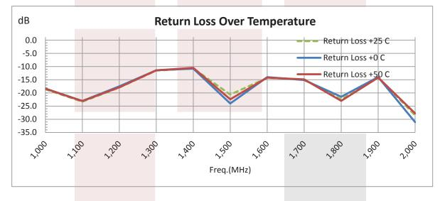
44 dB Gain High Power GaAs Amplifier at 8 Watt Psat Operating from 1 GHz to 3 GHz with 48 dBm IP3, SMA Input, SMA Output from Fairview Microwave is in-stock and available to ship same-day. All of our RF/microwave products are available off-the-shelf from our ISO 9001:2008 certified facilities in Allen, Texas. Fairview Microwave is RF on-demand.
