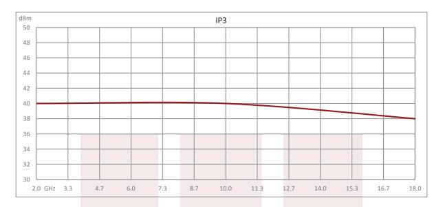
Medium Power Amplifier at 2 Watt P1dB Operating from 2 GHz to 18 GHz with 40 dBm IP3, SMA from Fairview Microwave is in-stock and available to ship same-day. All of our RF/microwave products are available off-the-shelf from our ISO 9001:2008 certified facilities in Allen, Texas. Fairview Microwave is RF on-demand.
