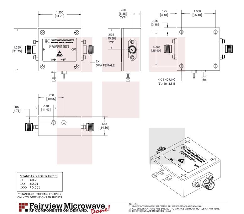
2 dB NF Low Noise Amplifier, Operating from 20 MHz to 4 GHz with 25 dB Gain, 18 dBm P1dB and SMA
