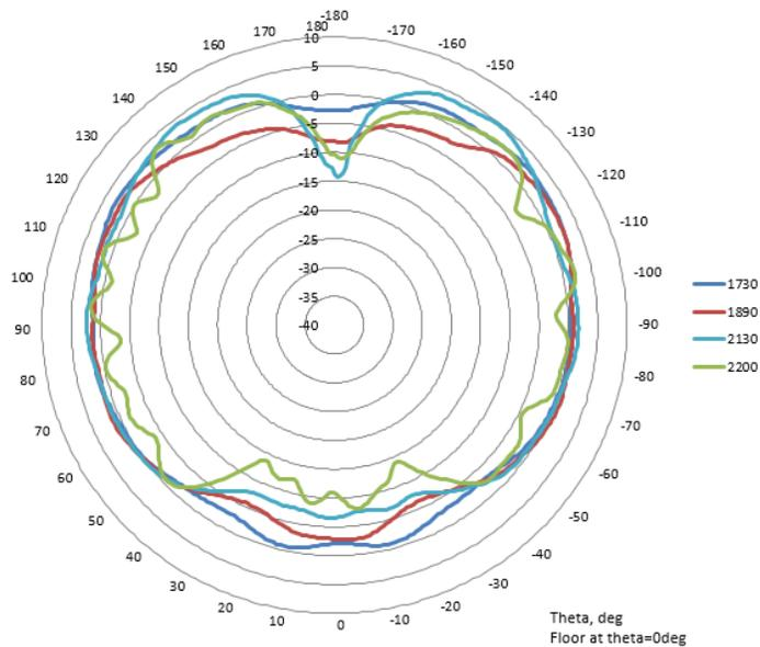
Mid band conical azimuth plane @ 45deg elevation
