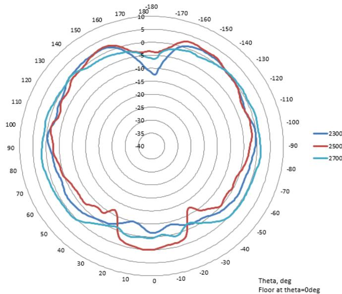
High band conical azimuth plane @ 45deg elevation
