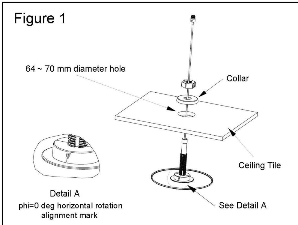
Note: Fiberboard ceiling tile is soft; tighten the nut just enough to hold the antenna firmly in place.
