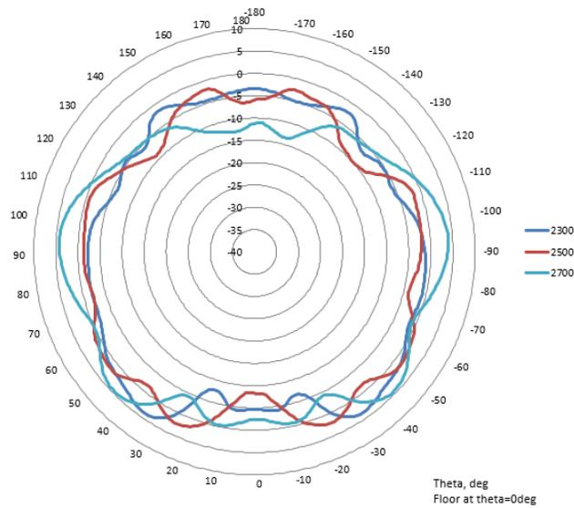
High band conical azimuth plane @ 45deg elevation
