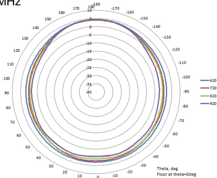
Low band conical azimuth plane @ 45deg elevation
