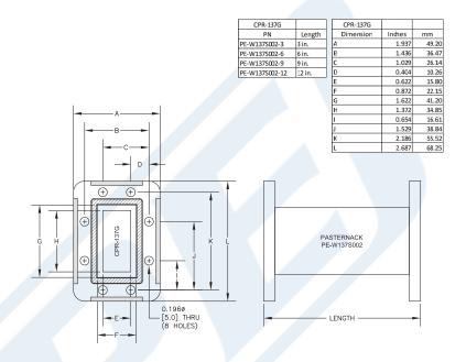
WR-137 Commercial Grade Straight Waveguide Section 12 Inch Length with CPR-137G Flange Operating from 5.85 GHz to 8.2 GHz from Pasternack Enterprises has same day shipment for domestic and International orders. Our RF, microwave and millimeter wave products maintain a 99% availability and are part of the broadest selection in the industry.
