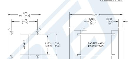
WR-112 Commercial Grade Straight Waveguide Section 12 Inch Length with UG-51/U Flange Operating from 7.05 GHz to 10 GHz from Pasternack Enterprises has same day shipment for domestic and International orders. Our RF, microwave and millimeter wave products maintain a 99% availability and are part of the broadest selection in the industry.
