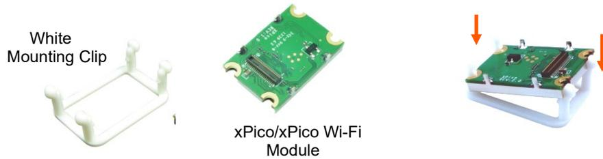
2. Push the legs of the white clip inward to secure the module to the clip.
