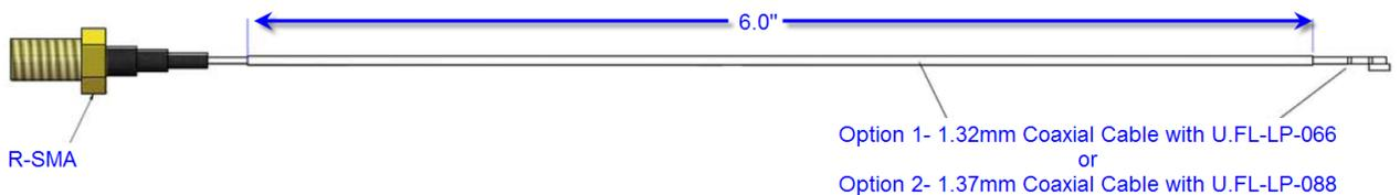
**Figure 2-5 U.FL to U.FL Cable (Lantronix Part Number 500-181-R)**
