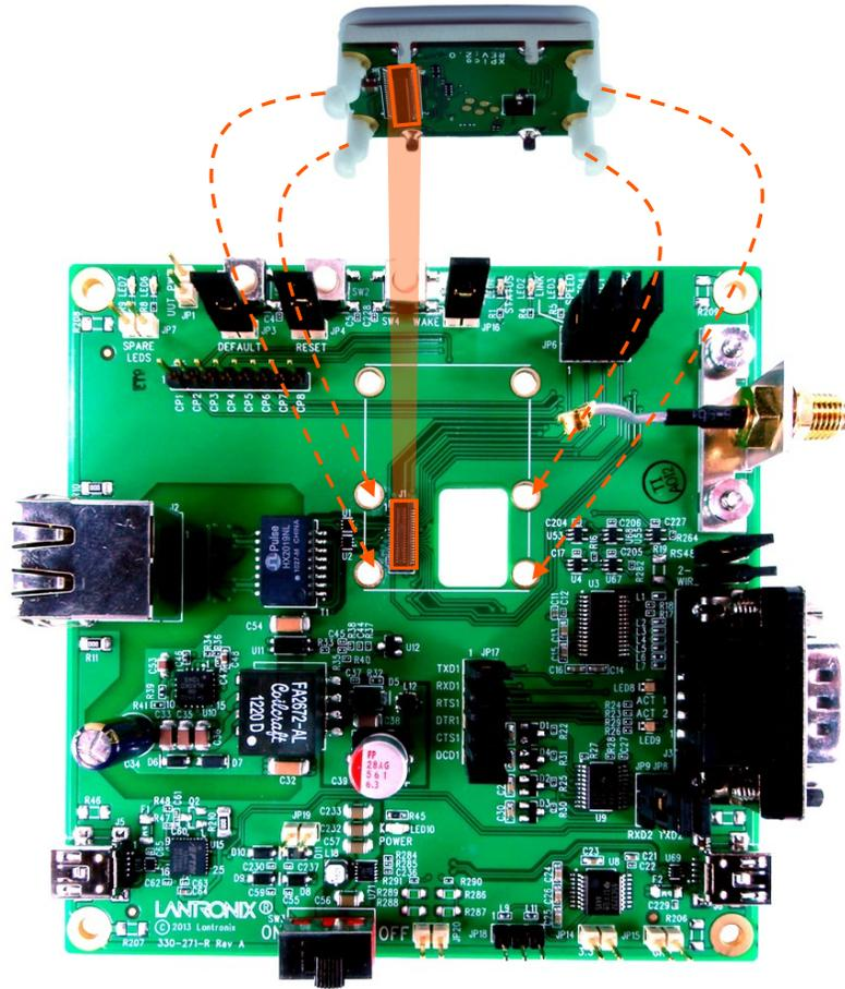
6. Insert the white clip legs furthest from the J1 connector first and gently push down on the xPico module above the J1 connector. Keep the module as level as possible during installation.
