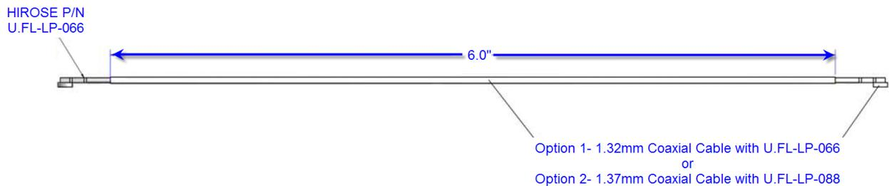
Figure 2-6 Reverse-SMA to U.FL(short) (Lantronix Part Number 500-182-R)
