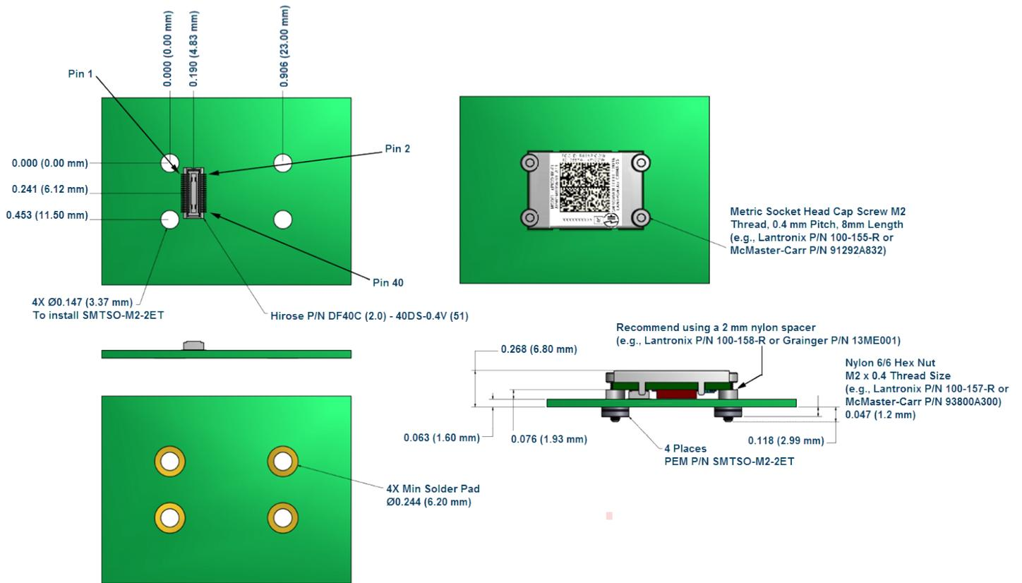
Figure 3-4 Hirose Connector Layout
