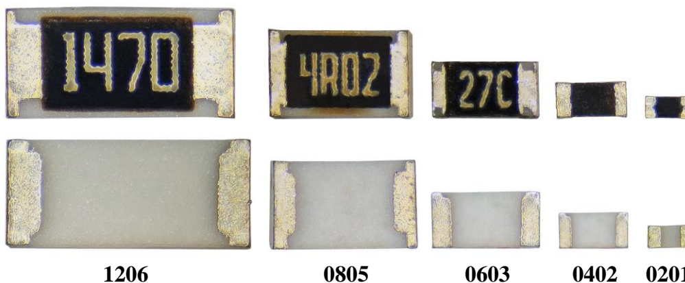
Figure 5. Resistor Marking Code
