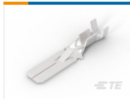
TE Part # 160451-3 FF 250 TAB 18-14AWG PB SILVER PL LP
