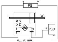
PS = Power Supply Z = Zero Adjust S = Span Adjust **Monitored Current** PLC = PLC Analog Input or Meter Input
