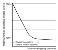
For a 5 A motor, the startup current would be approximately 30 A. The startup current would thus exceed the overload capacity of the K8AB-AS1 or K8AB-AS2 (150% of rated current for 1 s).
