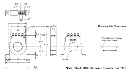
Note: The OMRON Current Transformer (CT) is designed to be used with the K8AB-AS3. Use terminals k and I for connections. (Terminals kt and It are not used.)
