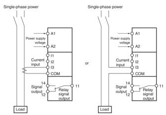
Note: The K8AB-AS3 is designed to be used in combination with the OMRON K8AC-CT200L Current Transformer (CT). The 24-VDC power supply type is a non-insulated power supply.
