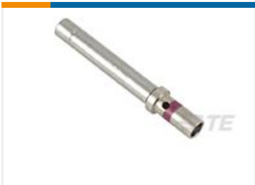
TE Part # 0462-005-20141 SOC, SOLID, SIZE 20, 16-18AWG, NI
