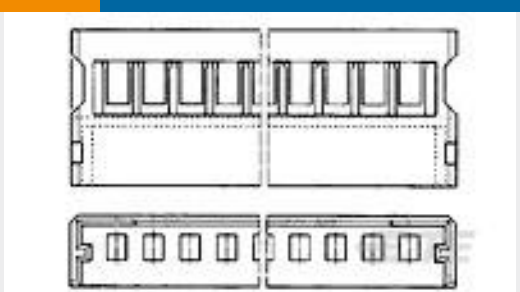
TE Part # 917572-4 1.5 B-T-W PLUG HSG 4P BLACK
